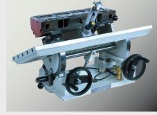
Rottler's patented dual axis leveling table and universal quick clamping system for surfacing/milling heads, blocks and manifolds with CBN and PCD tooling. The Rottler Dual Axis Leveling Table allows clamping of the head to be completed first, then the level adjusted in both directions simply by rotating the two hand wheels. Combined with Rottler's Dual Axis Level, any job can be clamped and leveled in seconds! This process results in minimal
