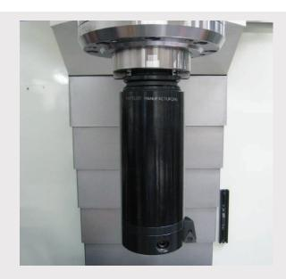
Rottler Boring and Sleeving Cutterhead installed in massive heavy duty EM69ATC Spindle.
