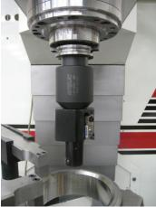
Special double diameter cutterheads allow both big end and small end to be bored in one automatic cycle. These cutterheads have pre-settable cartridges and can be adjusted in .0002" (.005mm).
