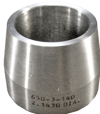
650-3-14D Locator, Cam, Small Block (2.1440 - 2.1450" bore) (54.45 - 54.48mm)
